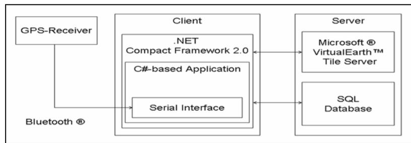
**Figure 1:** System Architecture. A classical Client-Server Architecture. The client in the human subject test is a *T-Mobile MDA Pro* Smartphone.
