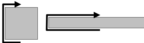
Fig. 3. Both cells have the same size but the right cell has a bigger form factor and creates the larger barrier.
